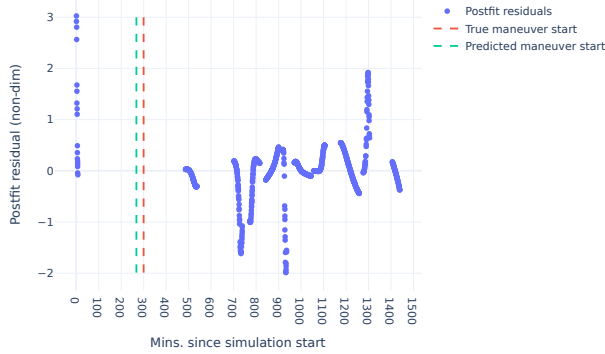
Figure 5: Example of a maneuver occurring in between tracking arcs, producing bad model predictions.
