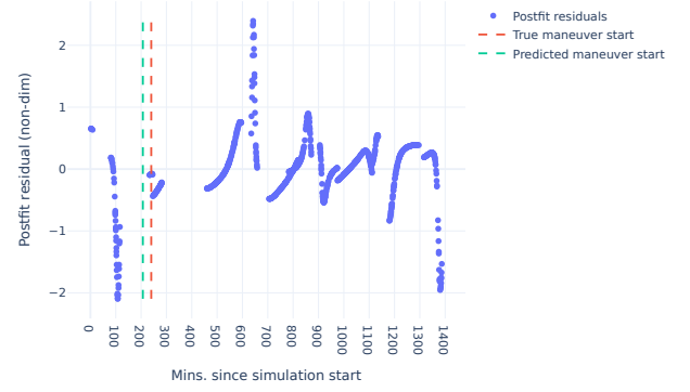
Figure 6: Example of sparse tracking around a maneuver, producing bad model predictions.
